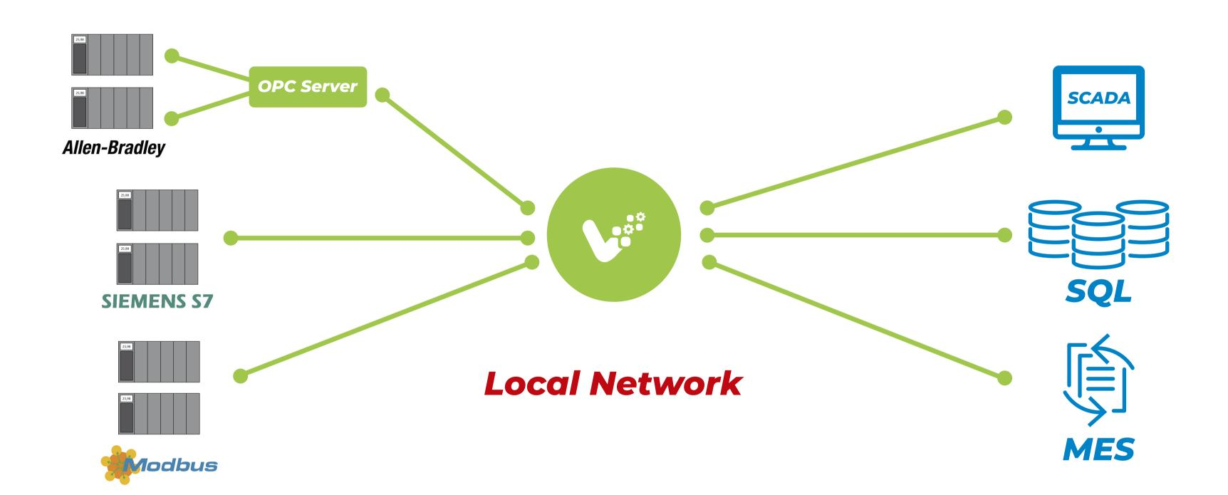
2) Linked Nodes between different networks. vNode can be configured to open the connection from the distributed Plant vNodes to the central IT vNode. Therefore there are no open ports at the Plant Firewalls.
